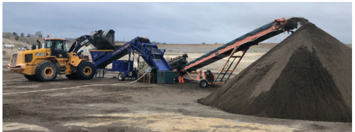
BioAgPhos ® in production, and the new BioAg screening plant in operation, at our solid products facility in Batesford, Victoria.
